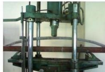
Fig. 6 Load applying on GFRP Leaf spring
